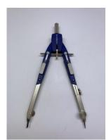
A compass can be expensive; we have a few extras in class. Purchase one according to your budget that has a sharp scribing point as we use this for making the halo. This suggested option has spring-loaded arms (gray pads beneath the adjustment bar) which make it easy to pull open to the right distance for large adjustment, while the wheel makes minor adjustments.
